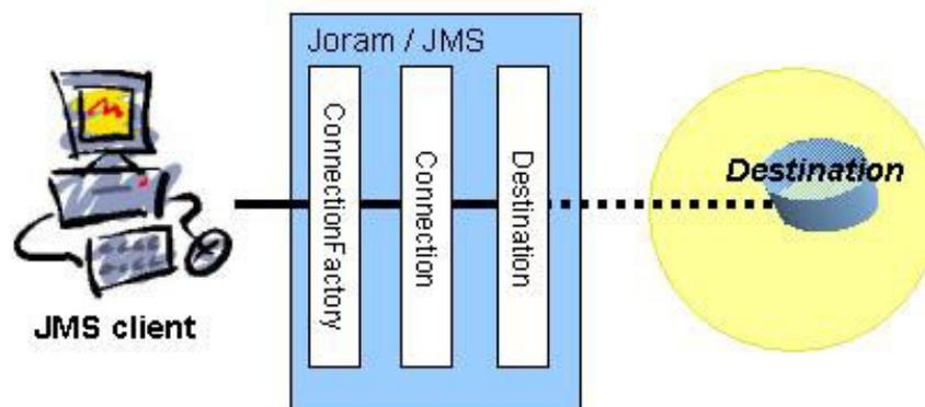
Figure 8. A client accessing a server destination “through” a standard Destination
