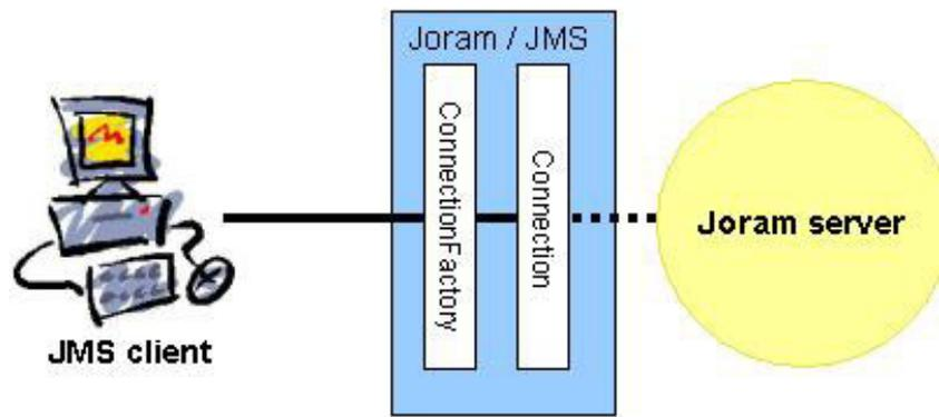
Figure 7. A client connected to a server “through” a standard `ConnectionFactory`
