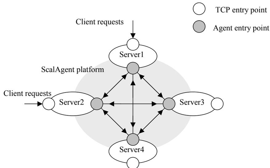
A new naming server is added into a JNDI configuration by assigning it one or more references of other servers already included into the configuration. When a naming server discovers another server, it sends to it an initialization notification containing its master copies and a list of the known servers. In this way a server discovers all the servers of a JNDI configuration.
