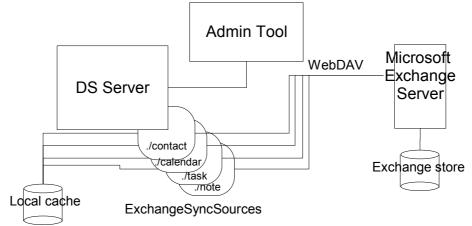
Figure 1 - Funambol Exchange Connector high level architecture
