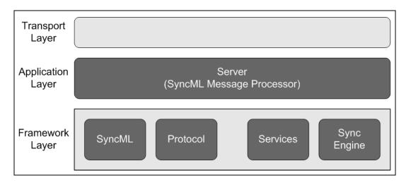
The Funambol core architecture is implemented in layers, as shown below:
