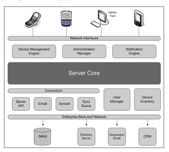
Funambol provides the following components around the server core:
