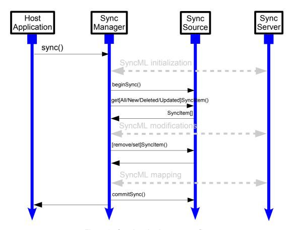
Figure 2 - Synchronization process flow
