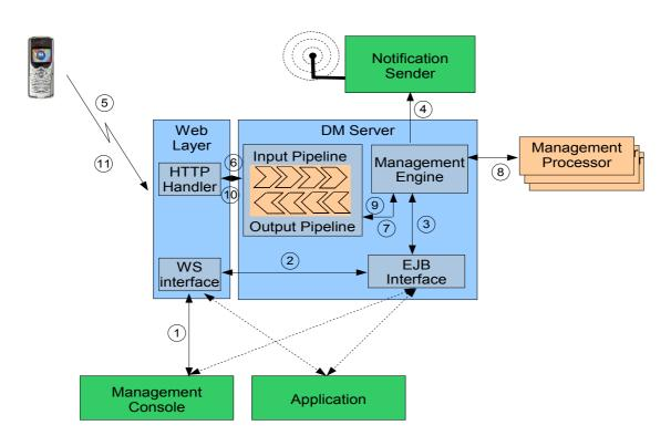
Figure 5 - Execution flow of an OMA DM request
