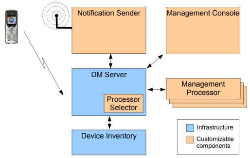
Figure 9 - Management engine architecture
