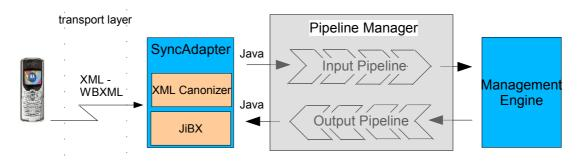
Figure 7 - Message processing architecture
