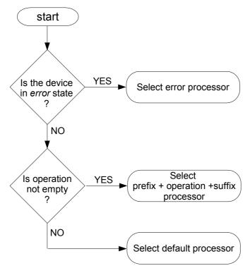
Figure 10 - OperationProcessorSelector selection flow chart
