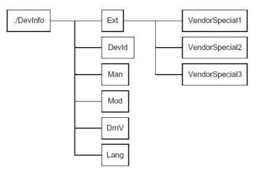
Figure 2 - Example of DM tree object mapping
