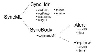
Figure 8 - sync4j.framework.core object tree example
