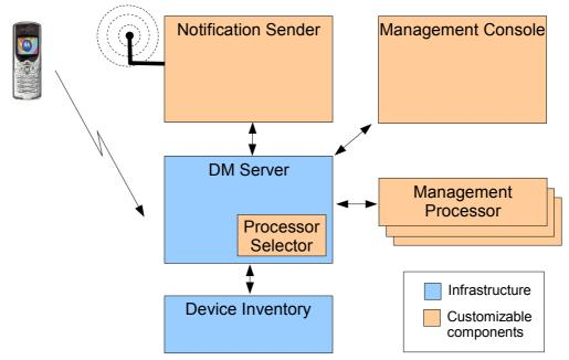
Figure 9 - Management engine architecture
