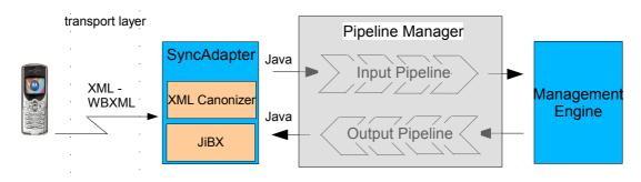
Figure 7 - Message processing architecture
