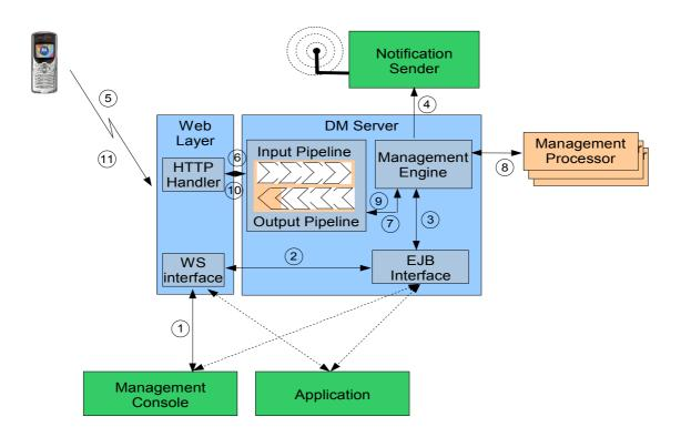
Figure 5 - Execution flow of an OMA DM request
