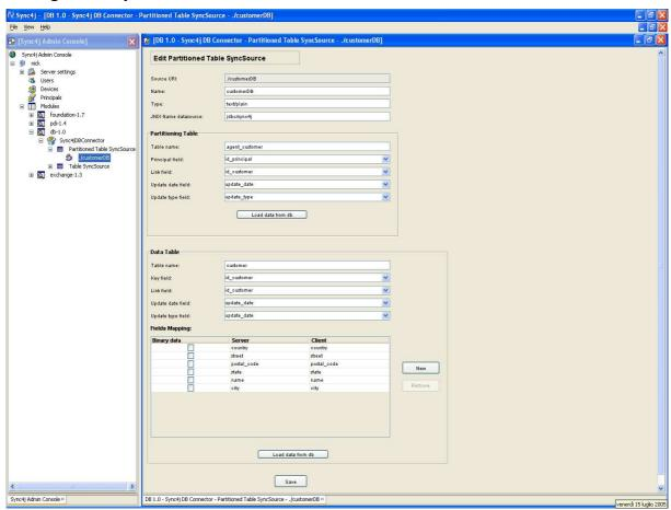
Figure 12 - The PartitionedTableSyncSource's configuration panel
