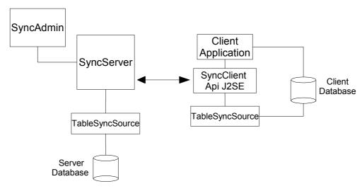
Figure 6 - Sync4j DB Connector high level architecture
