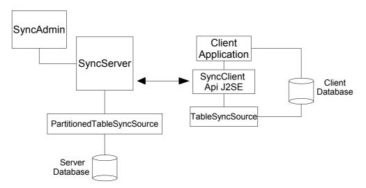
Figure 11 - Sync4j DB Connector high level architecture
