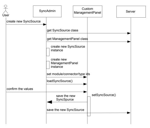
Figure 11 - SyncAdmin-ManagementPanel interaction diagram
