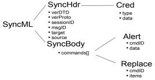
Figure 13 - sync4j.framework.core object tree example
