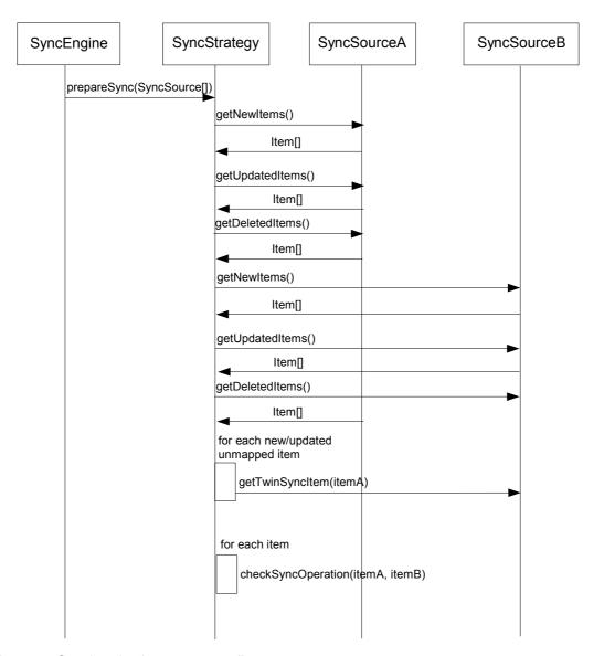
Figure 7 - Synchronization sequence diagram
