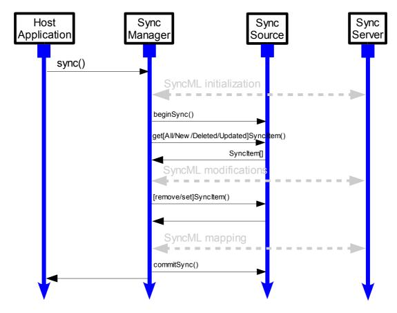
Figure 2 - Synchronization process flow
