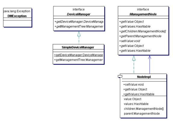
Figure 3 - SyncPlatform DM class diagram
