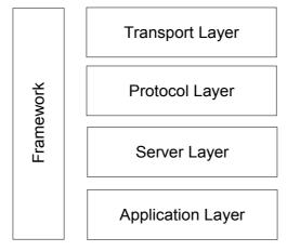
Figure 3 – DM Server layered architecture
