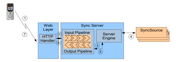
Figure 4 - Execution flow of an OMA DM request
