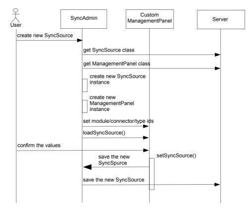
*Figure 11 - SyncAdmin-ManagementPanel interaction diagram* First of all, when the user right clicks on a SyncSource type and selects Add, few things happen:
