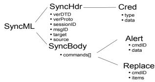
Figure 13 - sync4j.framework.core object tree example
