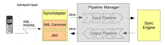
Figure 12 - Message processing architecture
