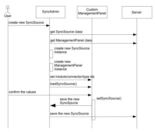
Figure 11 - SyncAdmin-ManagementPanel interaction diagram
